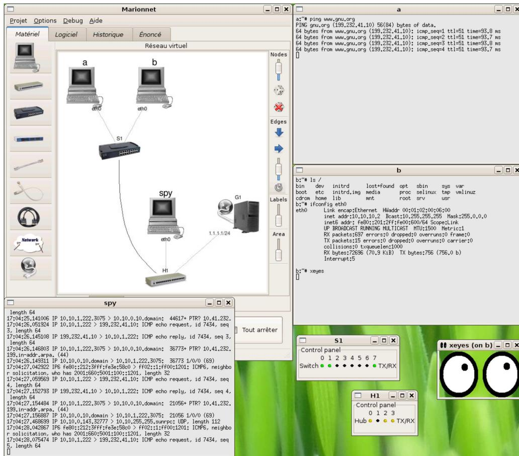
**Figure 7.** A very typical Marionnet session showing virtual machine terminals and device LED grids. The computer *a* is pinging a remote machine reachable via the gateway *G1*, *spy* is executing `tcpdump` observing *a*'s traffic, and *b* is running the graphical application `xeyes`. The network traffic between *b* and the host X server cannot be spied because of *ghostification*, as explained in subsection 4.9.1.
