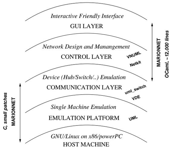
Figure 1. Emulation layers for a virtual network
